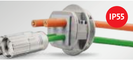
EMC Split cable gland for screw-in assembly, M32, M63 for cable diameters 2 to 33 mm EMC-KVT-DS 278 – 279
