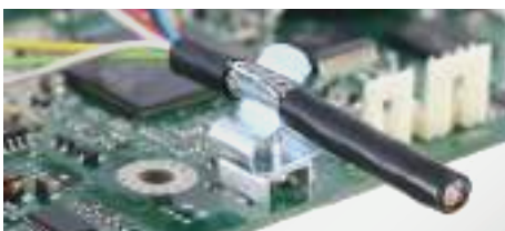
Shield clamps for printed circuit boards
