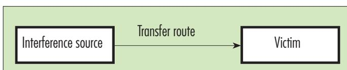
To combat cable carried interferences, mains filters or transient absorbers should be used.
